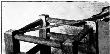
Fig. 225—Testing by Measuring
